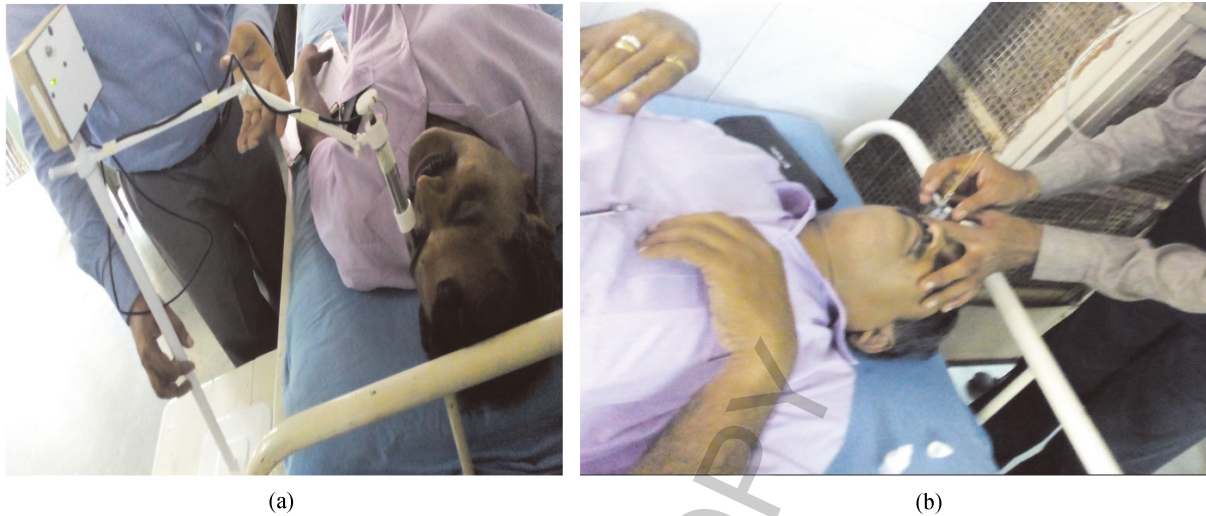
Fig. 2. (a) Testing of device on patient's eye; (b) Comparison of results with tonometer (Schiotz).
